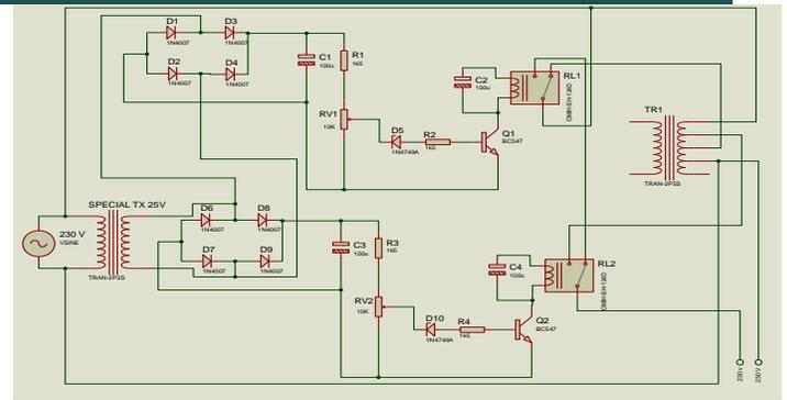
**Figure 3:** Circuit diagram of an automatic voltage stabilizer
