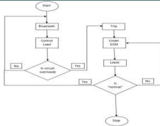
Figure 8: Flow chart For Automatic overload protector.
