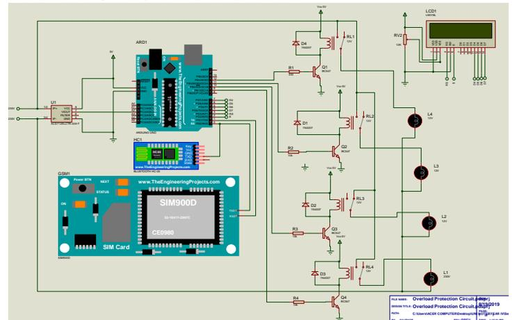
**Figure 4:** Circuit diagram of an automatic overload protector
