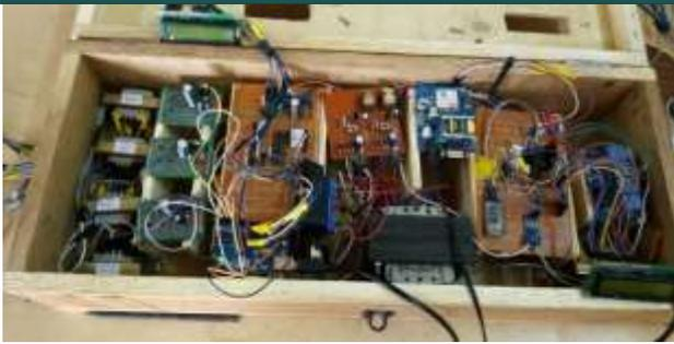
**Picture 1:** Automatic phase selector and overload protector implementation
