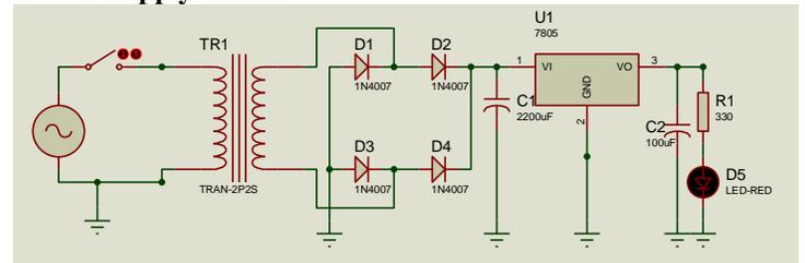
**Figure 5:** Regulated power supply circuit
