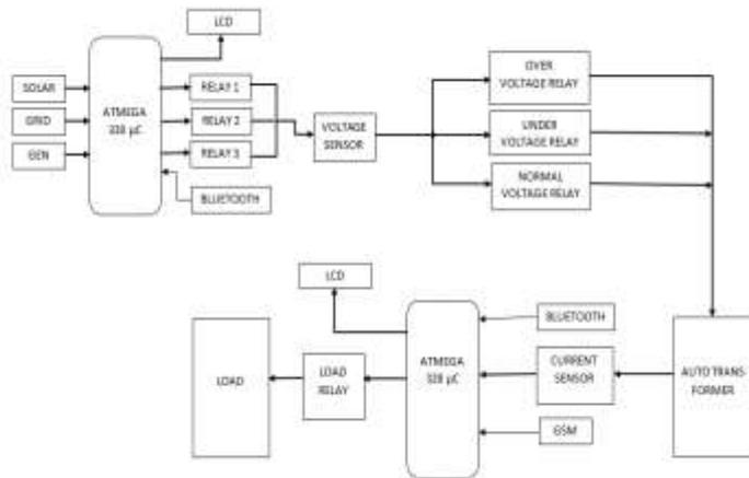
**Figure 1:** Block diagram of Automatic phase selector and voltage-Overload protection
