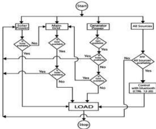
Figure 6: Flow chart for an automatic phase selector
