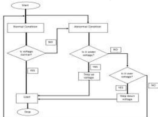
Figure 7: Flow chart For Automatic voltage stabilizer.
